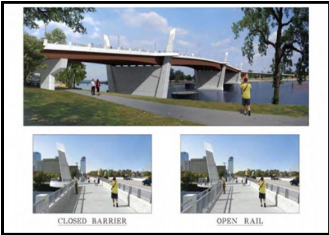
Figure 10. Plate Girder Design Bridge (Contemporary Design)
